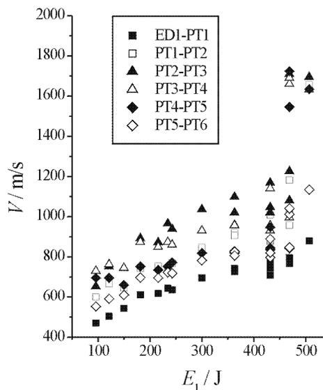
Fig. 5: Mean shock wave velocity at various measuring segments in a tube of Fig. 4 as a function of discharge energy. Fuel: *n*-hexane
