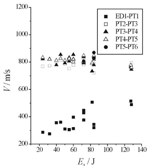
Fig. 3: Mean shock wave velocity at various measuring segments in a tube of Fig. 2 as a function of discharge energy. Fuel: *n*-hexane
