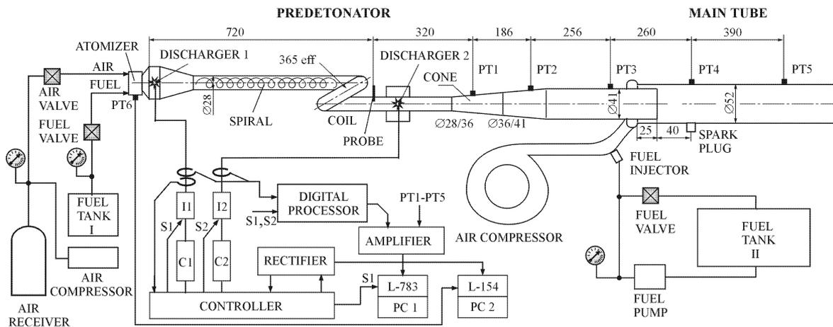
Fig. 1: Schematic of PDE demonstrator. Dimensions in millimeters
