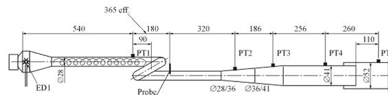
Fig. 7: Predetonator tube with the Schelkin spiral, single-loop coil, and transition section to a main tube
