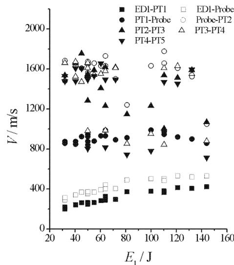
Fig. 8: Mean shock wave velocity at various measuring segments in a tube of Fig. 7 as a function of discharge energy. Fuel: *n*-hexane
