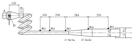
Fig. 4: Predetonator tube with three coils and a transition section to a main tube
