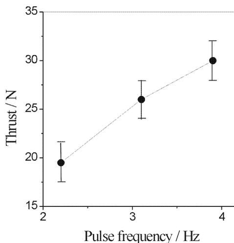
Fig. 12: Measured PDE thrust as a function of the operation frequency. Fuel: *n*-hexane
