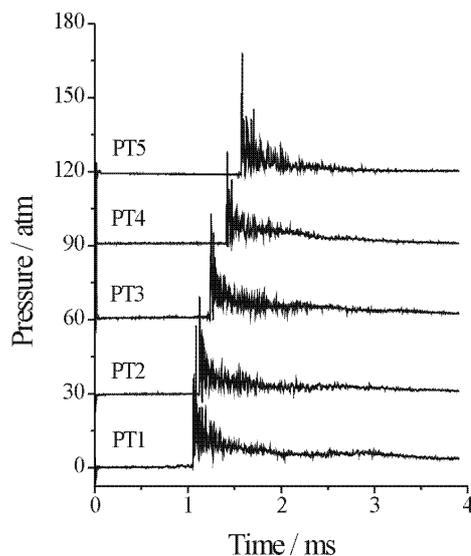
Fig. 6: Pressure histories registered by pressure transducers PT1 to PT5 in a tube of Fig. 4 at discharge energy of 507 J. Fuel: *n*-hexane
