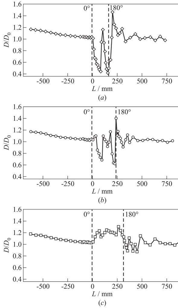
**Figure 4** Predicted normalized shock velocities along the internal wall (a), symmetry surface (b), and external wall (c) of the U-tube. The origin of the X-axis is located at the tube cross-section corresponding to the entrance to the U-bend. The region between the vertical dashed lines corresponds to the U-bend section
