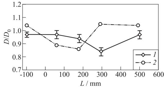
**Figure 5** Comparison of normalized predicted and measured shock velocities along the symmetry surface of the U-tube. The origin of the  $X$ -axis is located at the tube cross-section corresponding to the entrance to the U-bend: 1 — experiment and 2 — calculation
