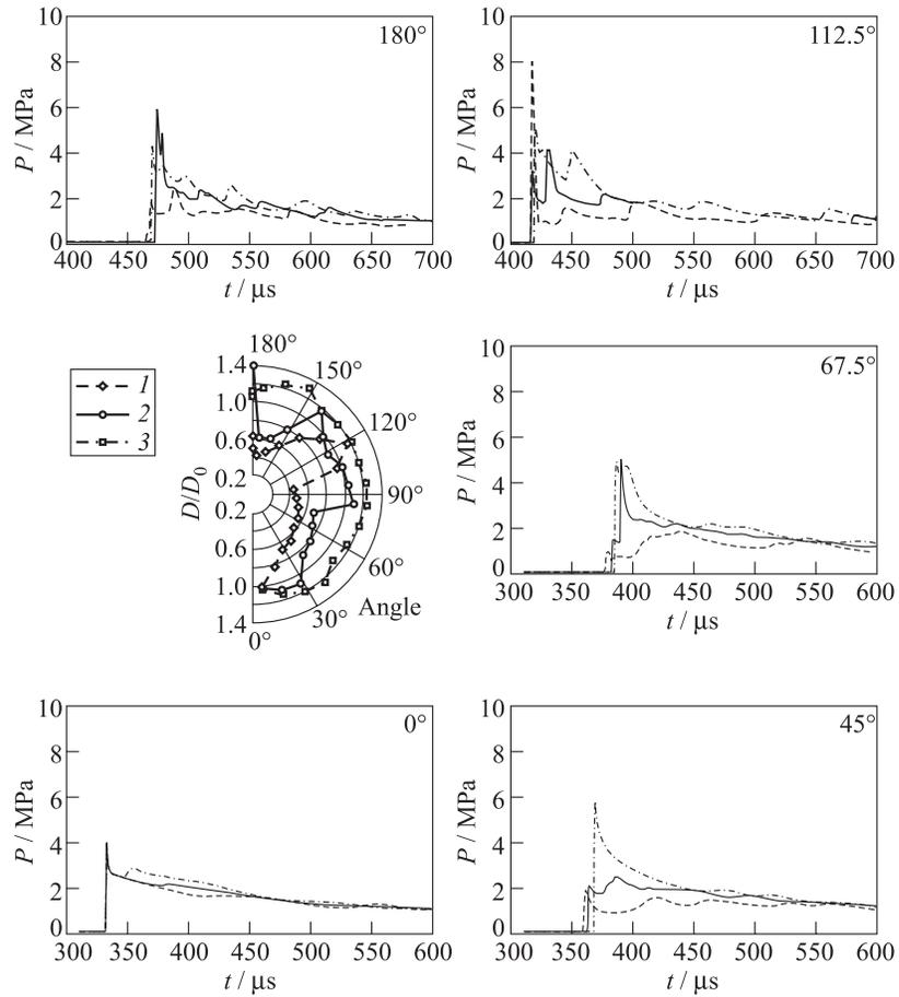
**Figure 6** Predicted normalized shock velocities in the U-bend as a function of the polar angle and the calculated pressure histories at different locations along the internal wall (1 and dashed curves), symmetry surface (2 and solid curves), and external wall (3 and dash-and-dot curves) of the U-tube and different polar angles (shown in the upper right corners)
