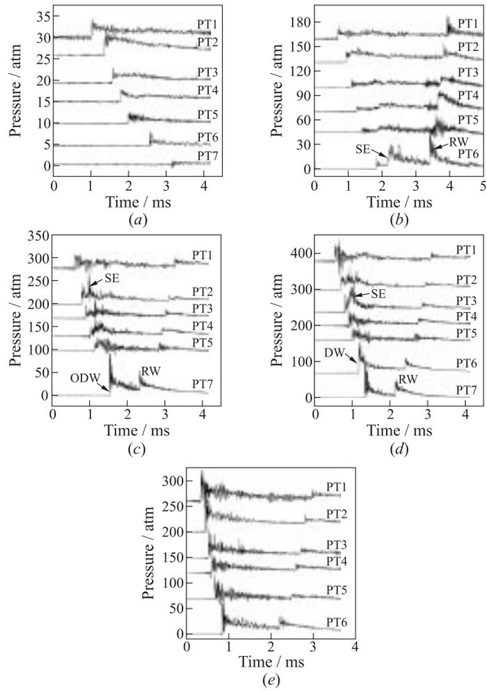
**Figure 3** Pressure records registered by the pressure transducers PT1 to PT7 in 5 representative runs with different mean shock wave velocities at the entrance to the U-bend (measuring segment PT1–PT2): (a) Run 1,  $V = 575$  m/s; (b) Run 2,  $V = 805$  m/s; (c) Run 3,  $V = 1083$  m/s; (d) Run 4,  $V = 1242$  m/s; and (e) Run 5,  $V = 1741$  m/s
