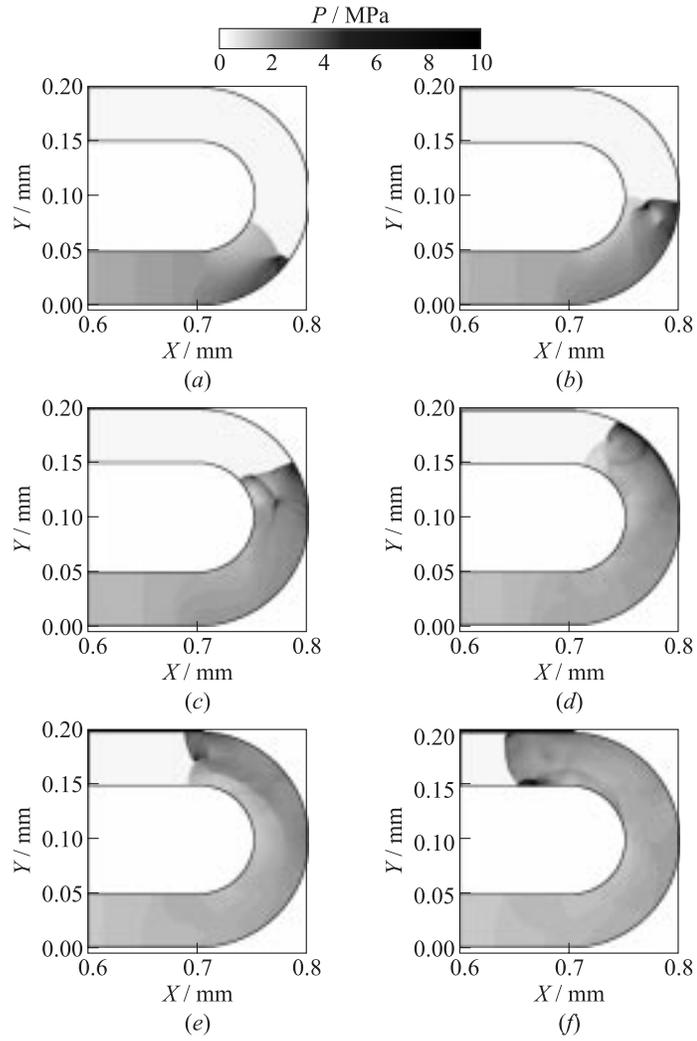
**Figure 7** Predicted evolution of the pressure field at propagation of a detonation wave through the U-bend. The snapshots (a) to (f) are plotted with a time interval of  $25 \mu\text{s}$
