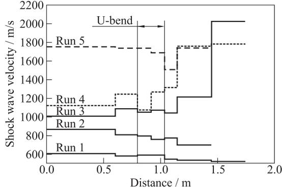
**Figure 2** Mean shock wave velocities at different measuring segments of the tube with the U-bend in 5 representative runs
