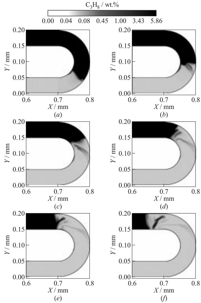
**Figure 8** Predicted evolution of the propane mass fraction field at propagation of a detonation wave through the U-bend. The snapshots (a) to (f) are plotted with a time interval of  $25 \mu s$
