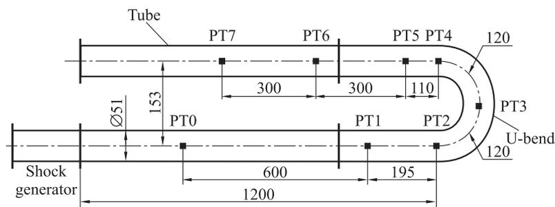
**Figure 1** Schematic of the experimental setup for the studies of detonation initiation and propagation in tubes with U-bends. Dimensions are in mm
