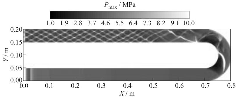
**Figure 9** Maximal pressure footprint at propagation of a detonation wave in the U-tube indicating the formation of a cellular detonation structure
