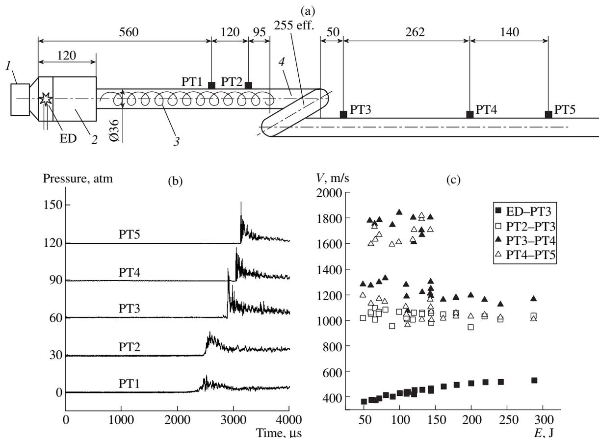
**Fig. 1.** (a) Schematic of an explosion tube 36 mm in diameter with a new element—a coil, (b) the pressure profiles recorded by transducers PT1–PT5 in an experiment with an ignition energy of  $E = 60$  J, and (c) the measured shock wave velocity in a drop *n*-hexane–air mixture over different measurement segments vs. ignition energy.
