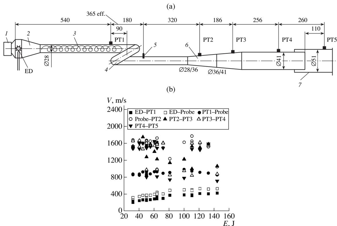
**Fig. 2.** (a) Schematic of an explosion tube 28 mm in diameter with a coil and a transition section to a tube 51 mm in diameter and (b) the measured shock wave velocity in a drop *n*-hexane–air mixture over different measurement segments vs. ignition energy.
