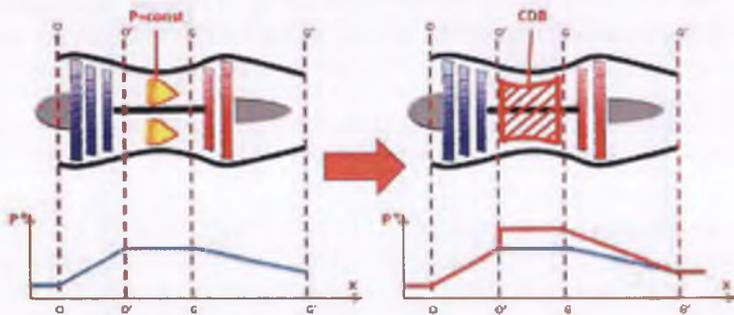
Fig. 1. Pressure-gain CDB concept for advanced gas-turbine power plant.
