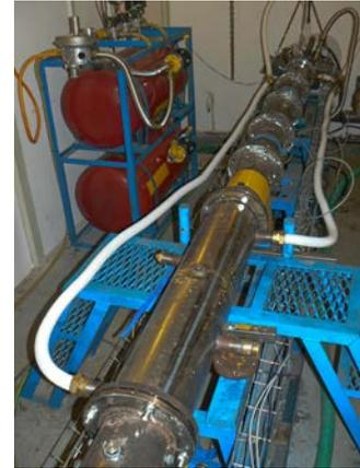
**Fig. 1.** Pulse detonation burner.
