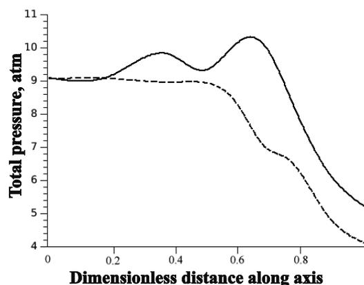
**Fig. 1:** Estimated distribution of the total pressure averaged over the cross section in the annular combustion chamber with detonation (solid curve) and deflagration (dashed curve)
