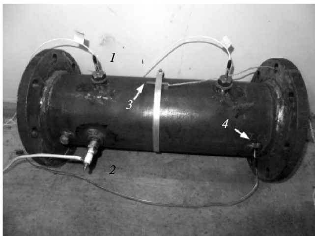
Fig. 3. Photograph of one of the sections of the burner duct: (1) pressure sensor, (2) ionization sensor, (3) heat target, and (4) thermocouples.
