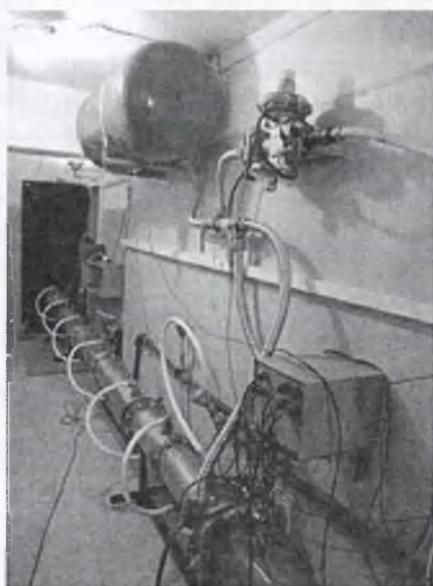
**FIGURE 1.** Pulsed detonation combustor operating on natural gas and air. The open end (far end) is immersed into a furnace.
