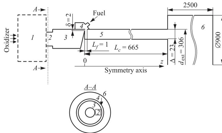
**Figure 1** Continuous detonation combustor of Lavrentyev Institute of Hydrodynamics [3]. Dimensions are in millimeters
