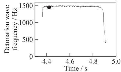
**Figure 6** Predicted (point) and measured (curve) [5] frequencies of detonation rotation in the CDC with air and hydrogen supply pressures of 4 and 18 atm
