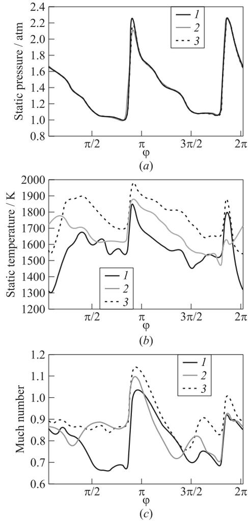
**Figure 4** Instantaneous distributions of static pressure (a), static temperature (b), and flow Mach number (c) vs. azimuthal angle  $\varphi$  along the outer (1) and inner (2) walls, and along the circumference in the middle of annular gap (3) at  $z = 665$  mm, at time 7.1 ms when steady-state mode of continuous-detonation combustion is already established in the CDC
