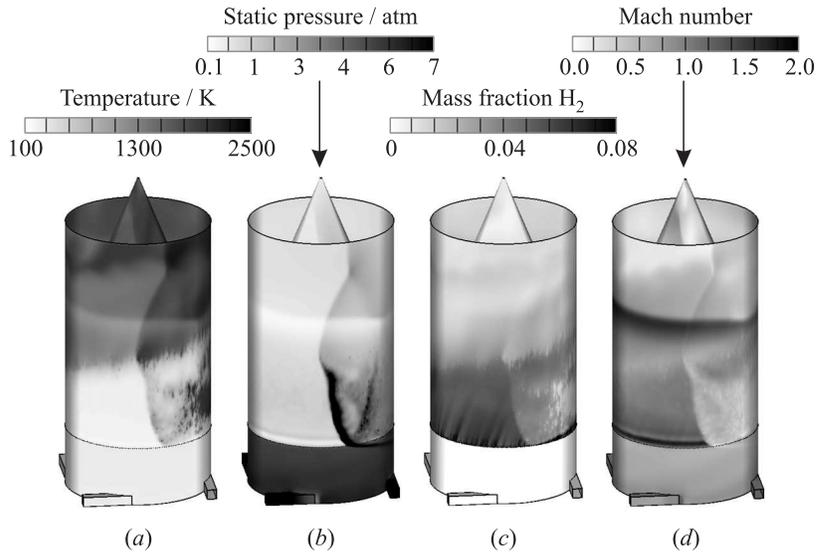
**Figure 5** Predicted snapshots of temperature (*a*), static pressure (*b*), mass fraction of hydrogen (*c*), and flow Mach number (*d*) near the outer wall of the CDC operating in the continuous detonation mode with one detonation wave at air and hydrogen supply pressures of 4 and 18 atm. Detonation propagates from right to left. Time: 7.65 ms after ignition
