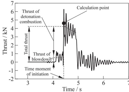
**Figure 7** Predicted (point) and measured (curve) [5] thrust produced by the CDC with air and hydrogen supply pressures of 4 and 18 atm
