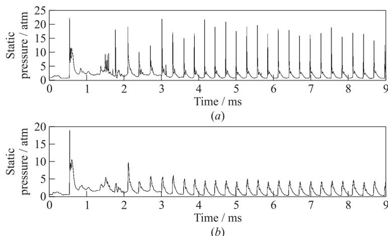
**Figure 3** Calculated time histories of static pressure in different CDC points: (a) at a point located on the outer wall at  $z = 40$  mm; and (b) at a point located on the inner wall at  $z = 40$  mm
