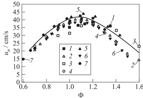
**Figure 4** Predicted (curve) and measured (points) laminar flame velocities in *n*-heptane–air mixture vs. equivalence ratio at 1 atm and 293 K: 1 — [14]; 2 — [15]; 3 — [16]; 4 — [17]; 5 — [18]; 6 — [19]; and 7 — [20]
