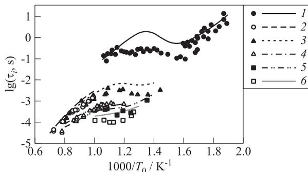
**Figure 1** Ignition delay vs. initial temperature for stoichiometric  $n$ -decane–air mixtures at different initial pressures (1 — 1.0 atm; 2 — 10; 3 — 12; 4 — 40; 5 — 50; and 6 — 80 atm) and temperatures. Curves — calculations and points — experiments [8–12]
