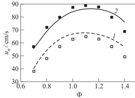
**Figure 5** Predicted (curves) and measured (points) laminar flame velocities in *n*-dodecane–air mixture vs. equivalence ratio at 1 atm and 400 K (1) and 470 (2): points — [21]
