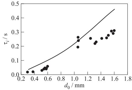
**Figure 8** Predicted (curve) and measured (points) [23,24] ignition delays of *n*-hexadecane drops vs. initial drop diameter at air temperature 1220 K and pressure 1 atm
