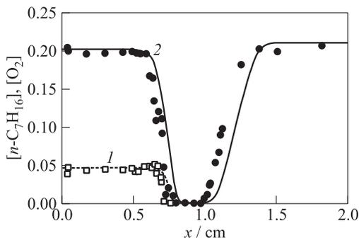
**Figure 7** Predicted (curves) and measured (points) [22] distributions of  $n\text{-C}_7\text{H}_{16}$  (1) and  $\text{O}_2$  (2) in the partially premixed counterflow flame of  $n$ -heptane-air and air
