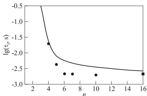
**Figure 2** Ignition delay vs. the number of carbon atoms  $n$  in the alkane hydrocarbon for stoichiometric  $C_nH_{2n+2}$ -air mixtures at initial temperature  $T_0 = 787$  K and initial pressure  $p_0 = 15$  atm. Curve — calculations and points — experiments
