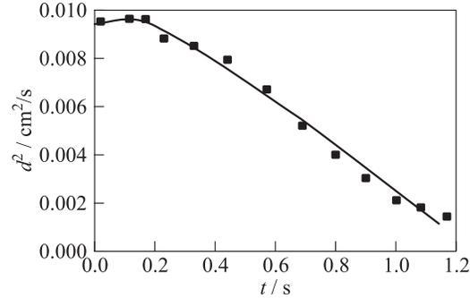
**Figure 9** Predicted (curve) and measured (points) [25] squared *n*-decane drop diameter vs. time. Initial drop diameter 0.91 mm, initial air temperature 1093 K, and initial air pressure 1 atm
