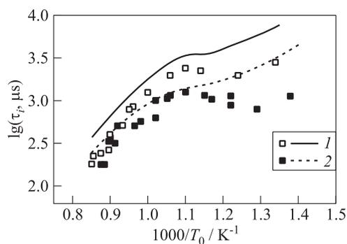
**Figure 3** Ignition delay vs. initial temperature for  $n$ -dodecane-air mixtures with equivalence ratios  $\Phi = 0.5$  (1) and  $1.0$  (2) at initial pressure  $p_0 = 20$  atm. Curves — calculations and points — experiments [9, 13]
