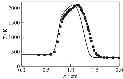
**Figure 6** Predicted (curve) and measured (points) [22] temperature distributions in the partially premixed counterflow flame of *n*-heptane–air and air
