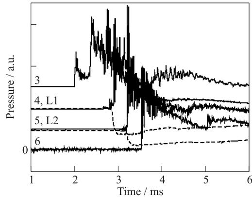
**Figure 2** Pressure profiles recorded by sensors 3–6 (solid curves) and luminescence intensity profiles recorded by photodiodes L1 and L2 (dashed curves) in experiment of series I
