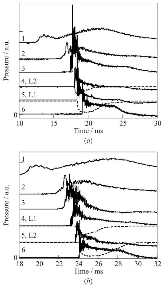
**Figure 3** Pressure profiles recorded by sensors 1–6 (solid curves) and luminescence intensity profiles recorded by photodiodes L1 and L2 (dashed curves) in experiments of series II (a) and III (b)
