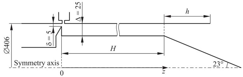
**Figure 1** Continuous detonation combustor. Dimensions are in millimeters
