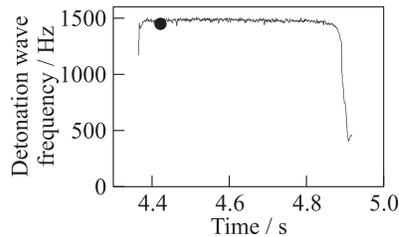
**Figure 4** Predicted (point) and measured (curve) frequencies of detonation rotation in the CDC of baseline configuration with air and hydrogen supply pressures 4 and 18 atm
