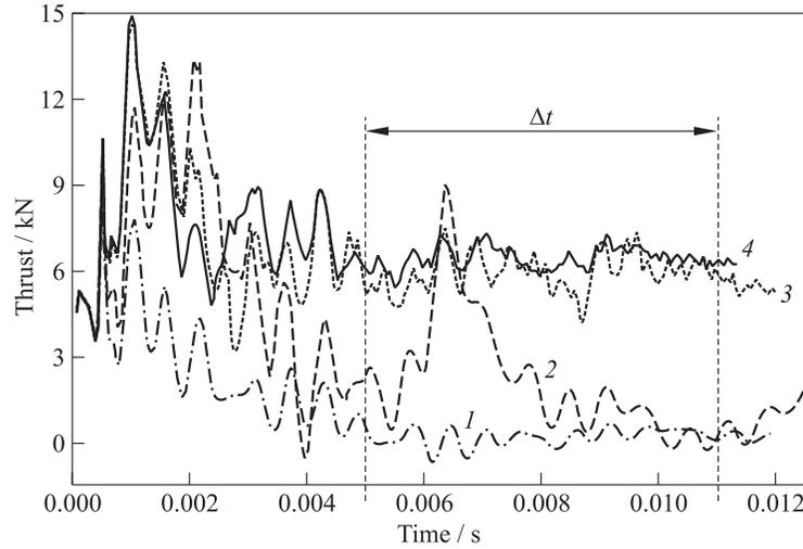
**Figure 7** Predicted time histories of thrust produced by the CDC at different overall equivalence ratios ( $\varphi$  is the fuel-air equivalence ratio and  $\Delta t$  is the time interval for estimating the CDC thrust): 1 —  $\varphi = 0.55$ ; 2 — 0.8; 3 — 1.0; and 4 —  $\varphi = 1.4$
