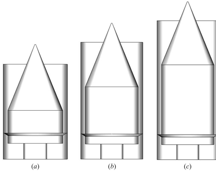
**Figure 6** Test cases with three different values of CDC height  $H$ : (a) 155 mm; (b) 310; and (c) 465 mm
