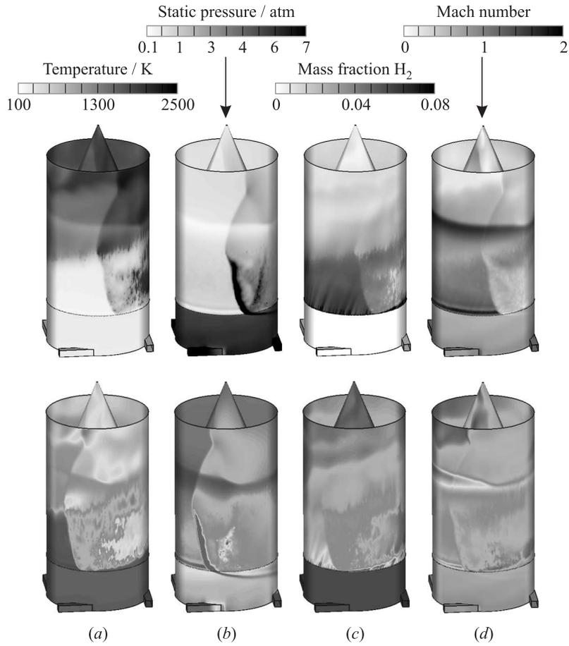
**Figure 3** Predicted snapshots of temperature (*a*), static pressure (*b*), mass fraction of hydrogen (*c*), and flow Mach number (*d*) near the outer wall of the CDC of baseline configuration operating in the continuous detonation mode with one DW at air and hydrogen supply pressures 4 and 18 atm. Detonation propagates from right to left: upper row — 7.65 ms after ignition, and lower row — 7.75 ms after ignition. (Refer color plate, p. XI.)
