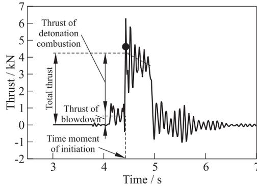
**Figure 5** Predicted (point) and measured (curve) thrust produced by the CDC of baseline configuration with air and hydrogen supply pressures 4 and 18 atm
