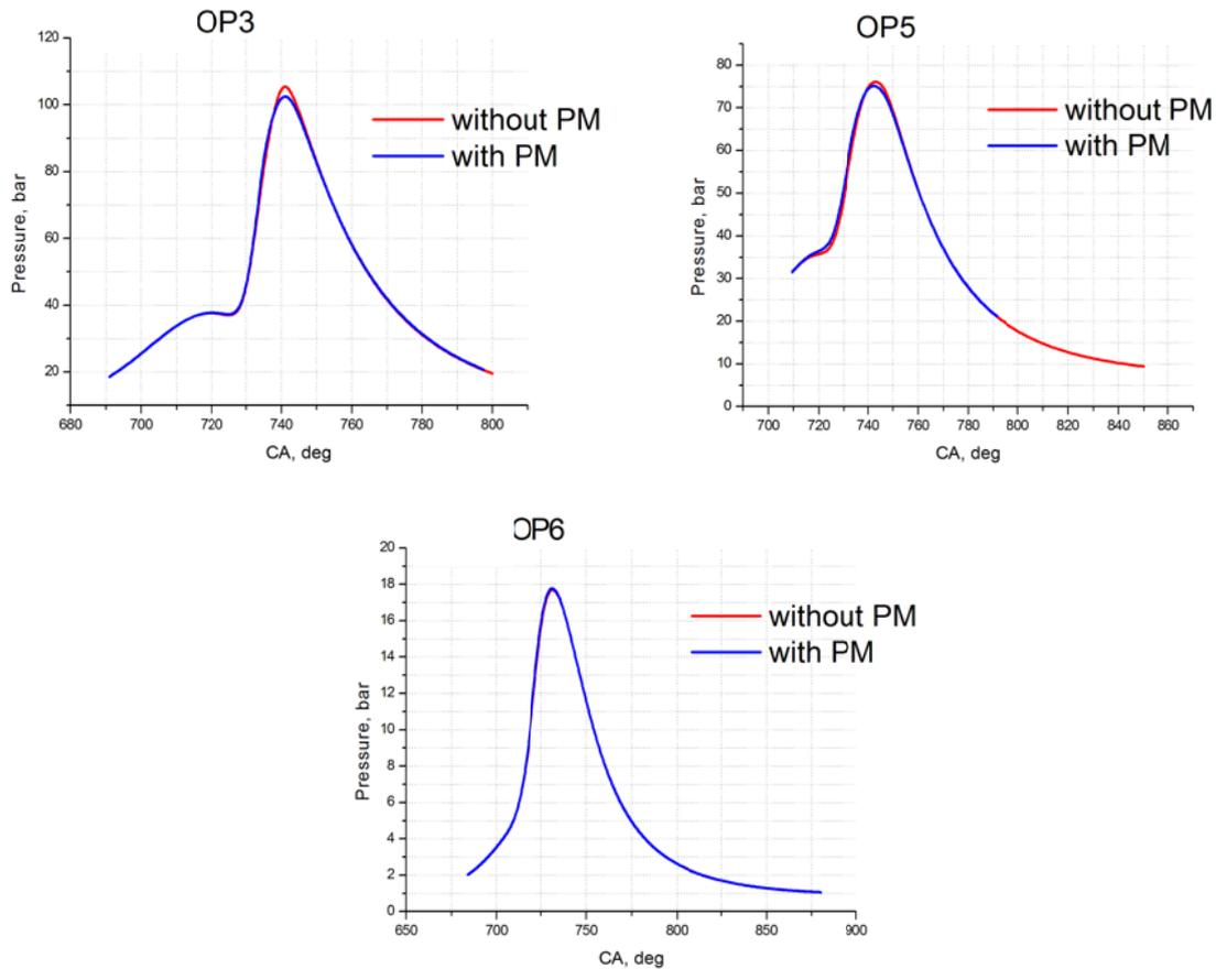
Figure 7: Comparison of predicted pressure histories obtained for three engine load points OP3, OP5, and OP6 with (blue) and without (red) activation of Particle method.
