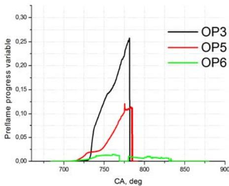
Figure 3: Predicted time histories of preflame reaction progress for three engine load points: OP3, OP5, and OP6.
