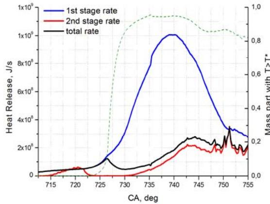
Figure 5: Predicted time histories of heat release due to cool-flame and hot-explosion reactions in the preflame zone for engine load point OP5. The dashed green curve shows the time history of the mass fraction of the preflame gas with temperature  $T > T^*$ , i.e. the preflame gas exhibiting the hot-explosion reaction stage.
