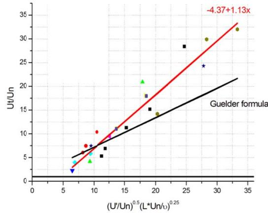
Figure 1: Engine test cases (points) and correlations for  $u_t / u_n$ : black line = Guelder correlation; red line = Engine correlation of Eq. (1).
