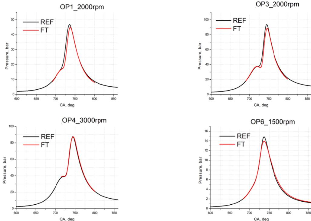
Figure 2: Comparison of predicted (red) and measured (black) pressure curves for different load points of one automotive engine with  $\alpha = 0.9$  in Eq. (1).
