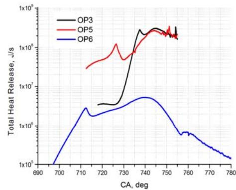
Figure 4: Predicted time histories of the rate of energy release in the preflame zone for three engine load points: OP3, OP5, and OP6.
