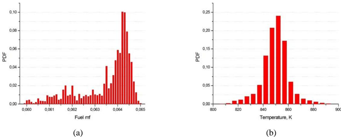
Figure 6: Predicted probability density functions of fuel mass fraction (a) and temperature (b) for a certain part of the engine combustion chamber.
