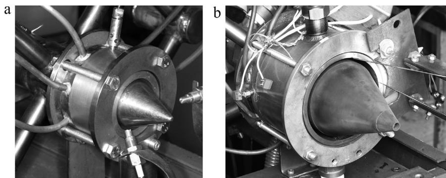
Fig. 1 – Photographs of two LRE prototypes with the annual combustor 50 mm (a) and 100 mm (b) in outer diameter.
