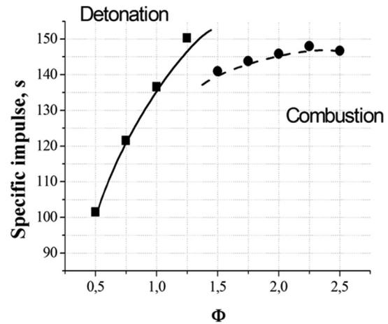
Fig. 6 – Specific impulse vs. equivalence ratio at a fixed fuel-mixture mass flow rate of 0.32 kg/s for the 100-mm-diameter LRE prototype.
