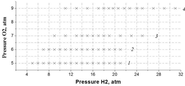
Fig. 4 – The matrix of 59 experiments with the 100-mm-diameter LRE prototype.
