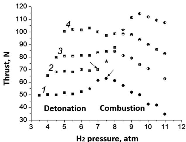
Fig. 2 – Thrust vs. hydrogen supply pressure at different oxygen supply pressures (series 1–3.5 atm, 2–4 atm, 3–4.5 atm, 4–5 atm) for the 50-mm-diameter LRE prototype.
