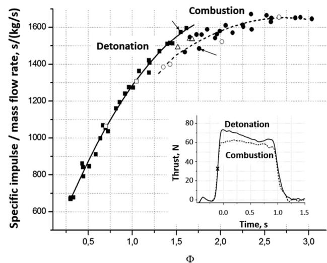
Fig. 3 – The ratio of specific impulse to fuel-mixture mass flow rate vs. mixture equivalence ratio for the 50-mm-diameter LRE prototype. Insert shows time histories of thrust at engine operation points marked by arrows: continuous-detonation mode (0.056 kg/s,  $\Phi = 1.55$ ) and continuous-combustion mode (0.053 kg/s,  $\Phi = 1.75$ ).
