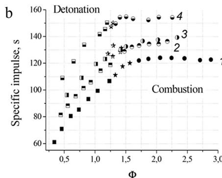
Fig. 5 – Experimental data for the 100-mm-diameter LRE prototype in terms of mass flow rate vs. equivalence ratio (a) and specific impulse vs. equivalence ratio (b).
