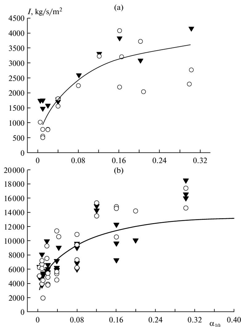
**Fig. 4.** Comparison of measured (symbols) and calculated (curves) dependences of the specific impulse of the bubbly liquid on the initial volumetric gas content for (a) relatively weak (with an amplitude of 0.05 MPa) and (b) strong ( $\approx 0.5$  MPa) SWs: the specific impulse of the bubbly liquid is determined from ( $\blacktriangledown$ ) the measured velocity of the contact surface and ( $\circ$ ) the measured velocity of the bubbles.
