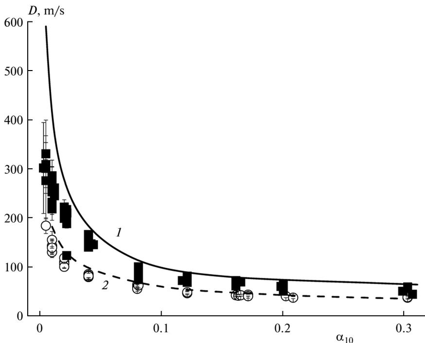
**Fig. 2.** Dependence of the SW velocity over the P5–P6 measuring segment on the volumetric gas content: (■) strong SW (with an amplitude of  $\approx 0.5$  MPa), experiment; (1) strong SW ( $\approx 0.5$  MPa), calculation; (○) weak SW ( $\approx 0.05$  MPa), experiment; (2) weak SW ( $\approx 0.05$  MPa), calculation.
