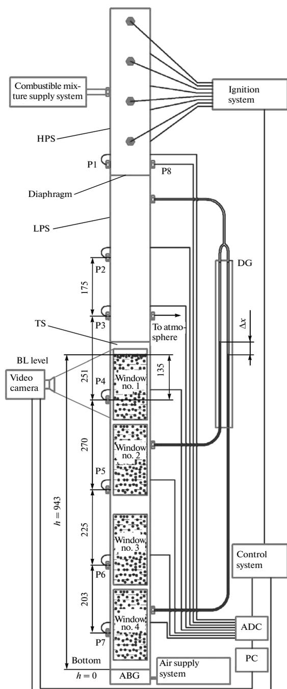
**Fig. 1.** Schematic diagram of the hydrodynamic shock tube: HPS, high-pressure section; LPS, low-pressure section; TS, test section, ABG, air, bubble generator, DG differential pressure gauge; P1–P7, PCB 113B24 piezoceramic overpressure sensors; P8, Kurant-DA tensorresistive absolute pressure sensor.
