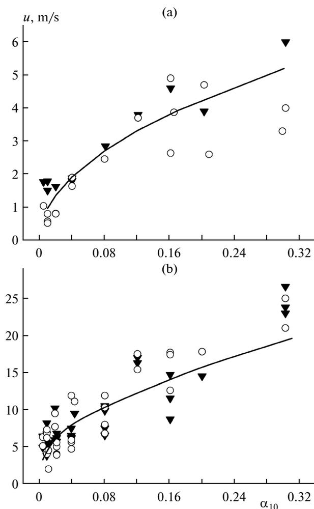
**Fig. 3.** Comparison of measured (symbols) and calculated (curves) dependences of the contact surface velocity and the velocity of air bubbles  $u$  on the initial volumetric gas content for (a) relatively weak (with an amplitude of  $\approx 0.05$  MPa) and (b) strong ( $\approx 0.5$  MPa) SWs: ( $\blacktriangledown$ ) contact surface velocity and ( $\circ$ ) velocity of the bubbles behind the SW front.
