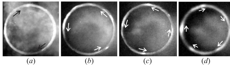
**Figure 6** High-speed video frames (200,000 frames/s) in the DLRE operating with two (a), three (b), four (c), and five (d) detonation waves
