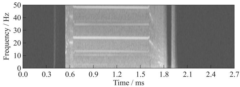
**Figure 5** Fast Fourier transform of the data obtained with the ionization probes for DLRE operation with five detonation waves
