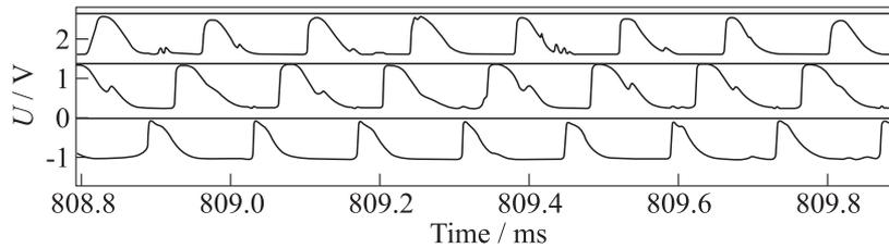
**Figure 4** Example of a record of continuous-detonation operation process with one detonation wave in NG–oxygen mixture
