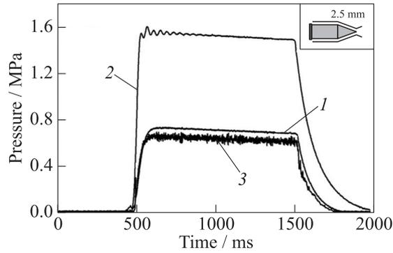
**Figure 3** Example of overpressure histories in oxygen (1) and NG (2) collectors and in the combustor (3) during firing a DLRE of the configuration shown in the insert
