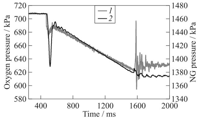
**Figure 2** Experimental pressure histories in oxygen and NG receivers: 1 — pressure of gaseous oxygen; and 2 — pressure of NG
