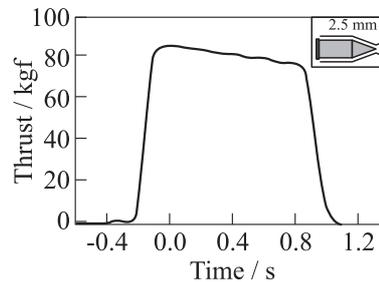
**Figure 8** Example of the measured time history of DLRE thrust
