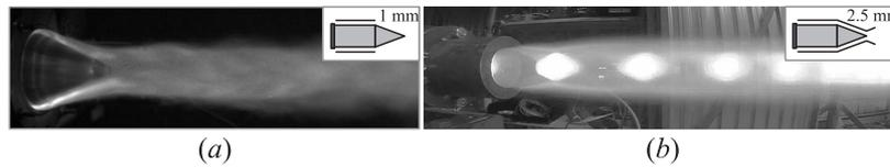
**Figure 7** Photos of exhaust jets in firing tests of DLRE without (a) and with (b) CD nozzle extension
