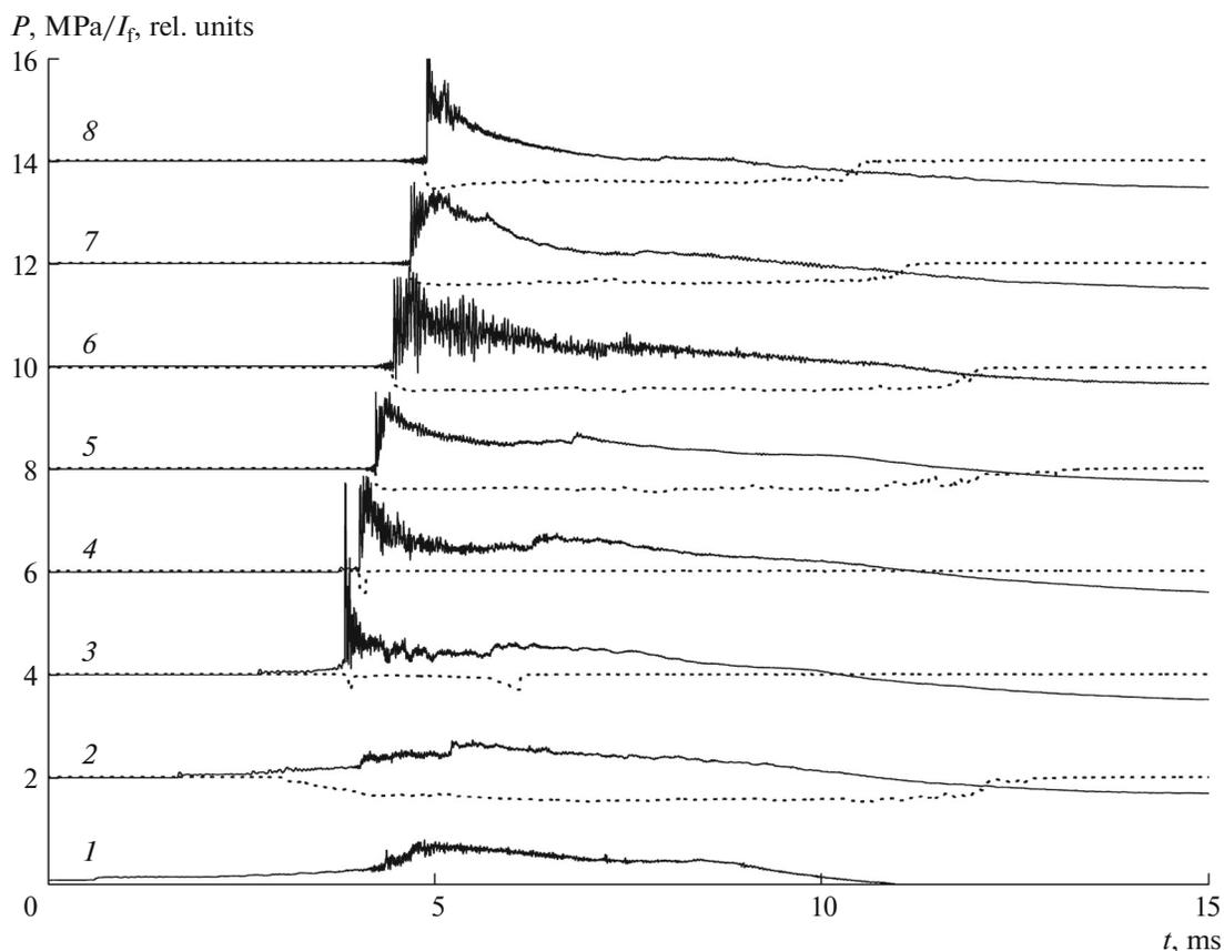
Fig. 2. Readings of pressure gauges (continuous curves) and photodiodes (dashed curves) in test 2.
