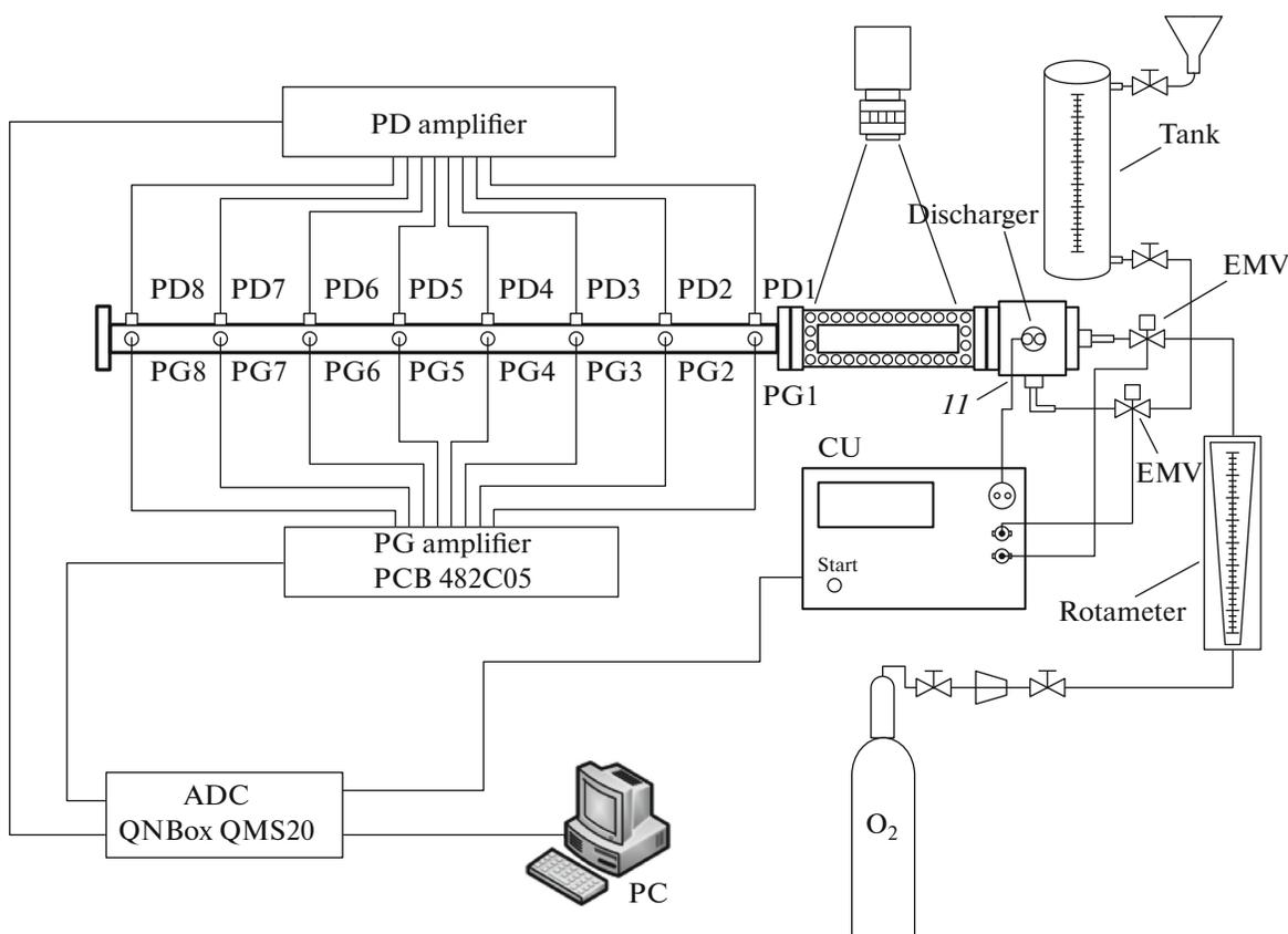
Fig. 1. Scheme of experimental setup with optical section.
