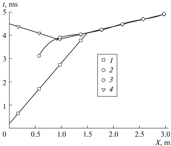
**Fig. 3.** Experimental  $x(t)$  diagram of test 2: (1) weak shock wave from the ignition source, (2) flame front, (3) detonation wave, and (4) retonation wave.
