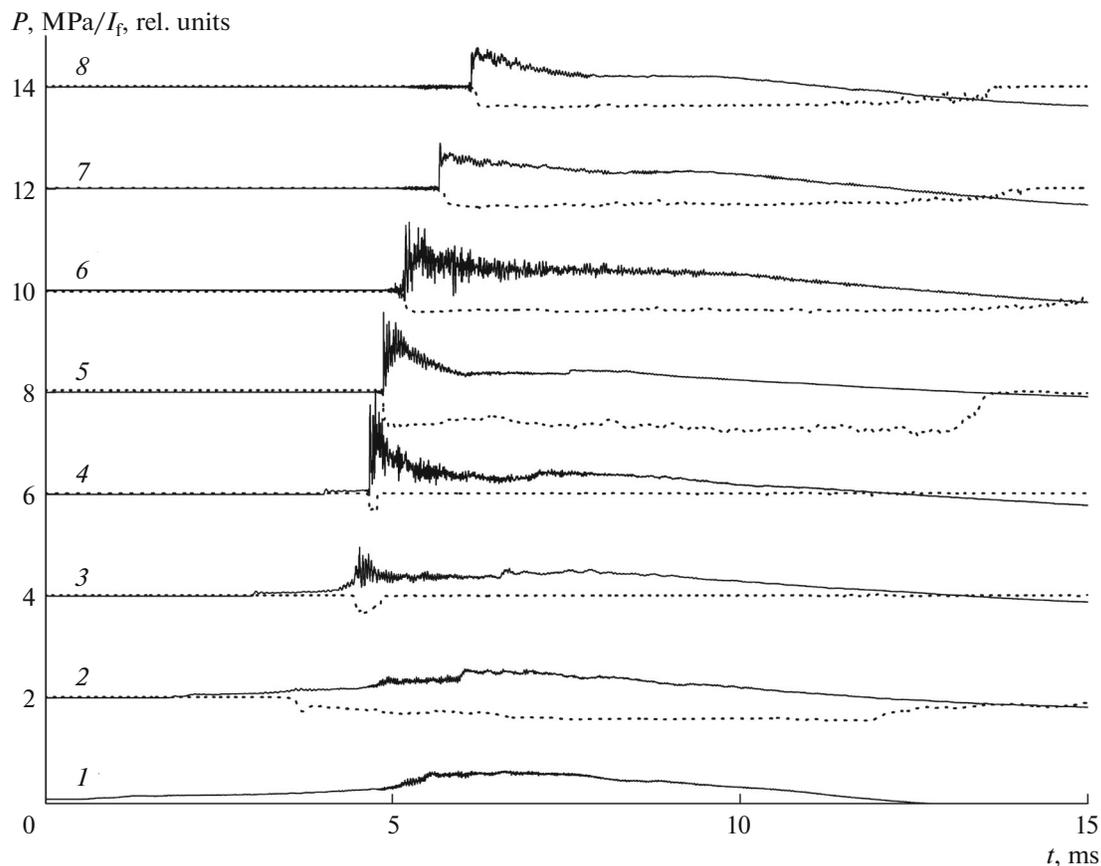
**Fig. 4.** Readings of pressure gauges (continuous curves) and photodiodes (dashed curves) in test 1.
