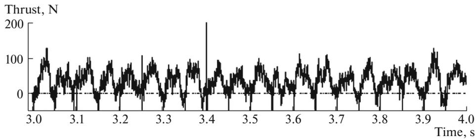
Fig. 3. Example of the oscillogram of the thrust force generated by PDH EP at an approach water stream velocity of 10 m/s and an operation frequency of 20 Hz.
