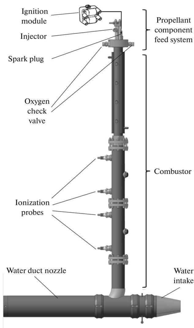
Fig. 1. Schematic of PDH EP.
