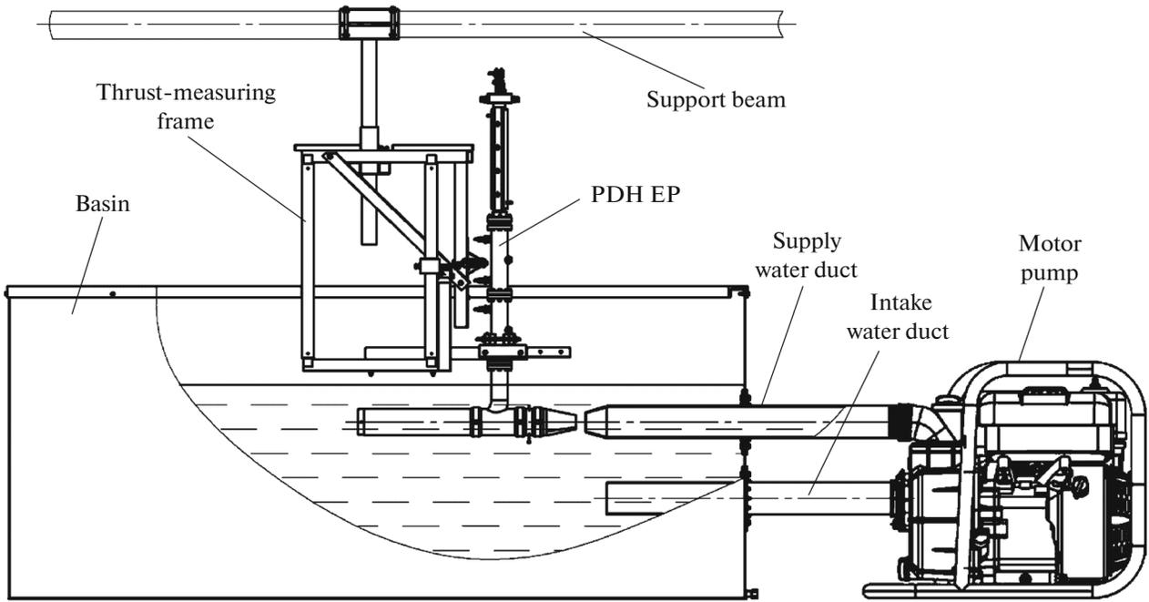
Fig. 2. Schematic of test stand.
