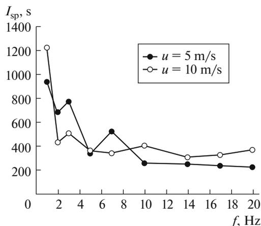
Fig. 4. Measured dependences of the specific impulse of PDH EP on the operation frequency at two values of the approach water stream velocity.
