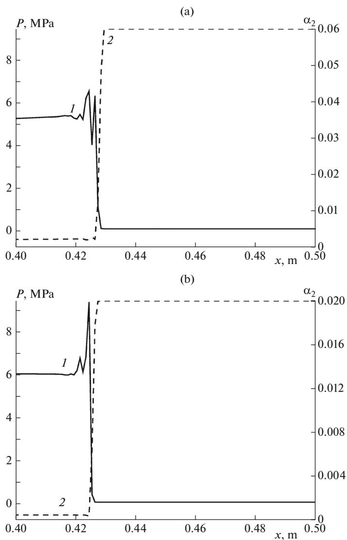
**Fig. 7.** Structure of the pressure wave in water with air bubbles in cross section 5 at initial gas volume fractions of (a) 6 and (b) 2%: (1) pressure and (2) gas volume fraction.
