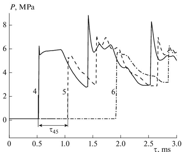
**Fig. 3.** Examples of calculated time histories of pressure in the cross sections in which the P4–P6 sensors are mounted (cross sections 4–6) for an initial gas volume fraction of 6%:  $\tau$ , time;  $\tau_{45}$ , time it takes for the pressure wave front to travel the distance between cross sections 4 and 5;  $x_{45}$ , distance between cross sections 4 and 5;  $D_{45} = x_{45}/\tau_{45}$  is the pressure wave velocity between cross sections 4 and 5.
