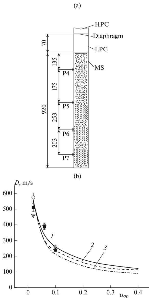
**Fig. 2.** Comparison of the results of the calculations with our experimental data: (a) experimental setup (dimensions in millimeters); (b) calculated pressure wave velocities as a function of the initial gas volume fraction in water with acetylene–oxygen mixture bubbles (curves) in the (1) P4–P5, (2) P5–P6, and (3) P6–P7 measuring segments and experimental data (symbols) obtained in the same segments: (■) P4–P5, (○) P5–P6, and (▽) P6–P7.
