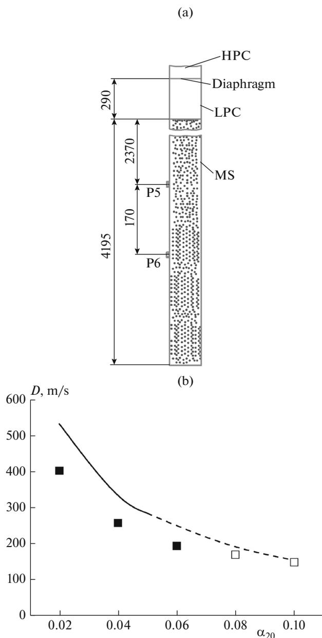
**Fig. 1.** Comparison of the results of the calculations with experimental data from Ref. [7]: (a) experimental setup (dimensions in millimeters); (b) calculated (curve) and measured (squares) pressure wave velocities as a function of the initial gas volume fraction in water containing acetylene–oxygen mixture bubbles.
