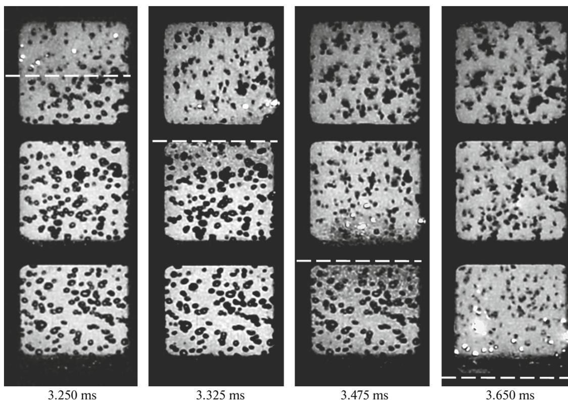
**Fig. 5.** Video shots of SW propagation in the reactive bubbly medium at  $\alpha_{20} = 2\%$  and  $P_{0, \text{HPC}} = 0.6$  MPa. Time is counted from the ignition point. Frame dimensions,  $160 \times 448$ ; recording speed, 40000 FPS. The white dashed lines indicate SW front positions.
