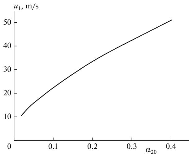
**Fig. 8.** Calculated maximum liquid velocity as a function of the initial gas volume fraction behind the detonation-like pressure wave front in the P5–P6 measurement segment.
