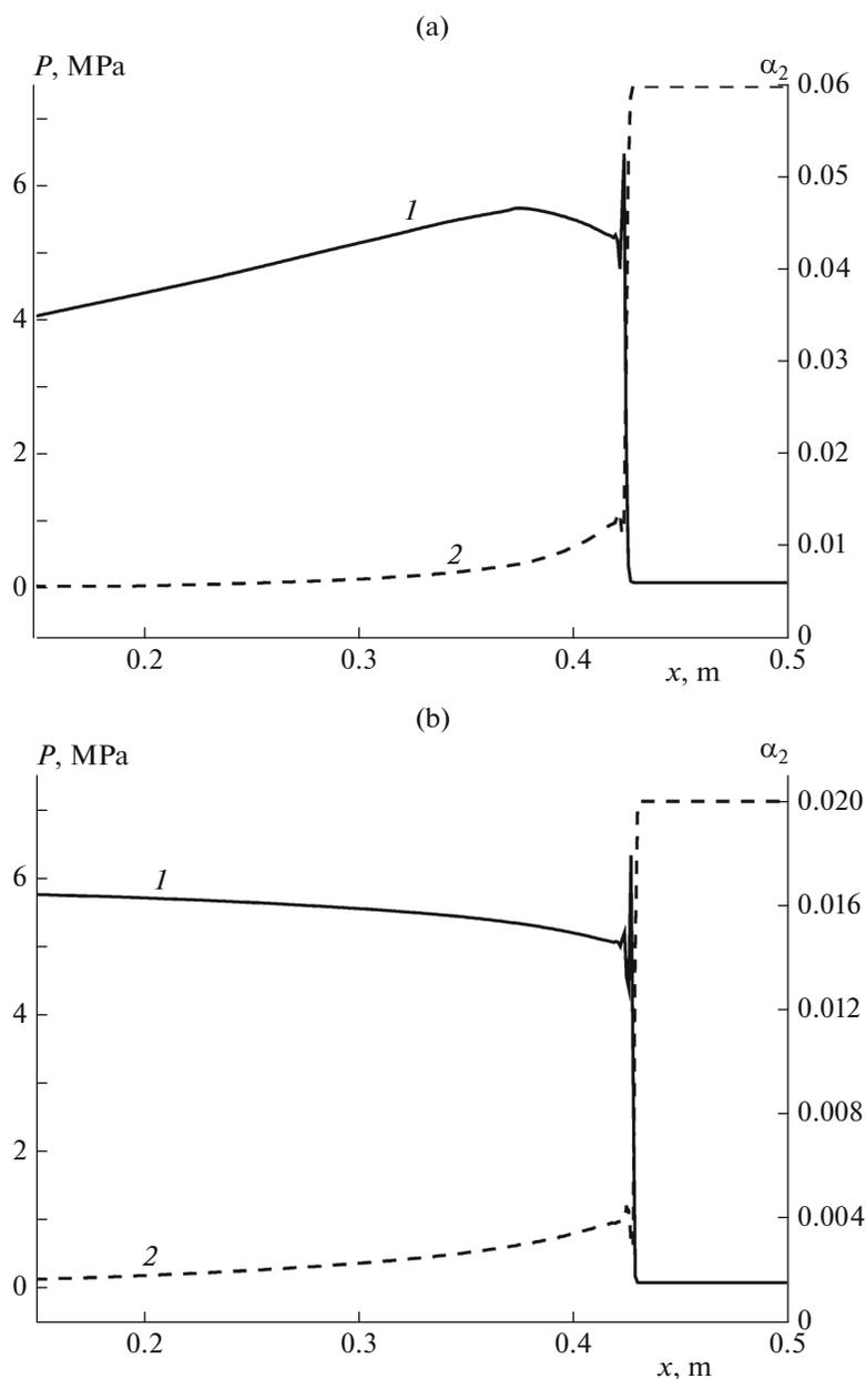
**Fig. 6.** Structure of the bubble detonation wave in cross section 5 at initial acetylene–oxygen mixture volume fractions of (a) 6 and (b) 2%: (1) pressure and (2) gas volume fraction.
