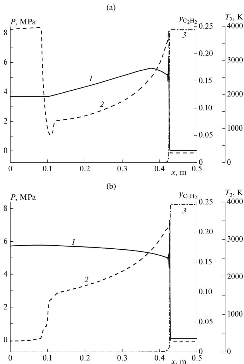
**Fig. 4.** Structure of the supersonic pressure wave in cross section 5 for initial gas volume fractions of (a) 6 and (b) 2%: (1) pressure, (2) bubble temperature, and (3) acetylene mass fraction in the bubble.
