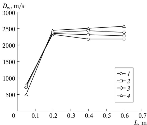
**Fig. 4.** Example of the measured dependences of the detonation wave velocity on the traveled distance in four successive pulses at an operating frequency of the setup of 10 Hz.
