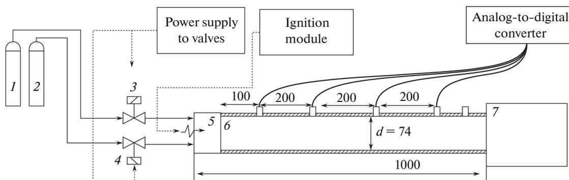
**Fig. 1.** Schematic of experimental setup: (1, 2) oxygen and natural gas cylinders, (3, 4) controlled valves, (5) spark plugs, (6) detonation tube, and (7) buffer tank. Dimensions are in millimeters.
