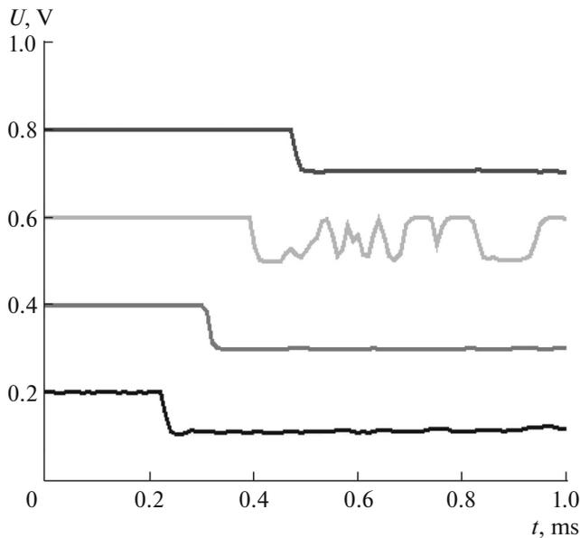
Fig. 2. Example of the ionization probe signal readings in a single pulse.
