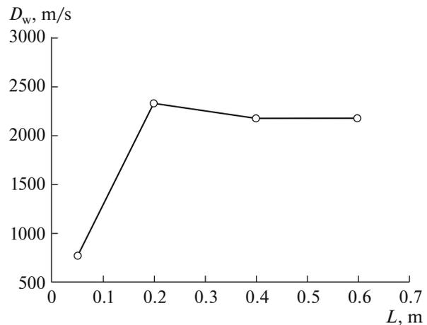
Fig. 3. Example of the measured dependence of the detonation wave velocity on the traveled distance in a single pulse.
