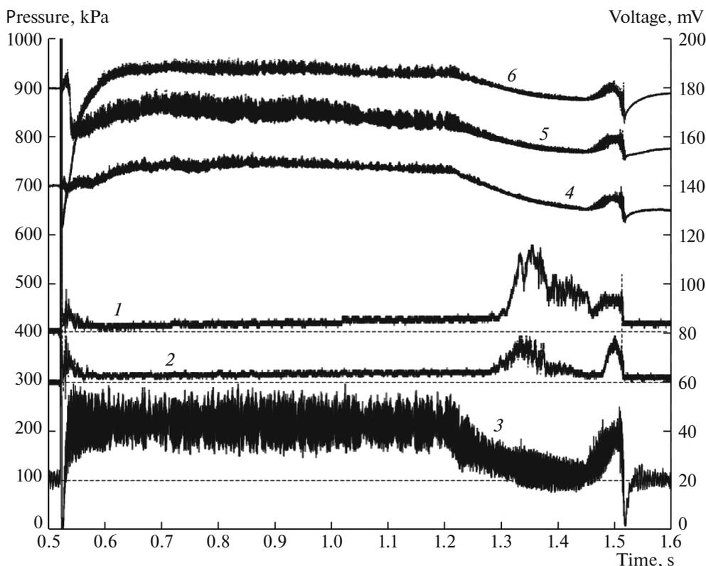
**Fig. 2.** Readings of (1, 2) the photosensors, (3) the static pressure sensor in the combustor, and (4–6) the pressure pulsation sensors in one of the firing tests.
