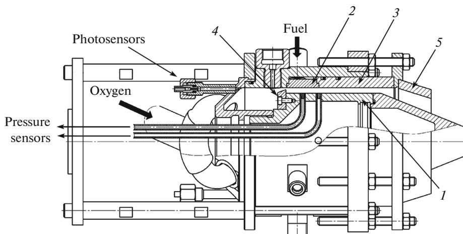
**Fig. 1.** Schematic of DRE: (1) center body, (2) porous ring liner, (3) hold-down impermeable ring liner, (4) hot side plate, and (5) convergent nozzle.
