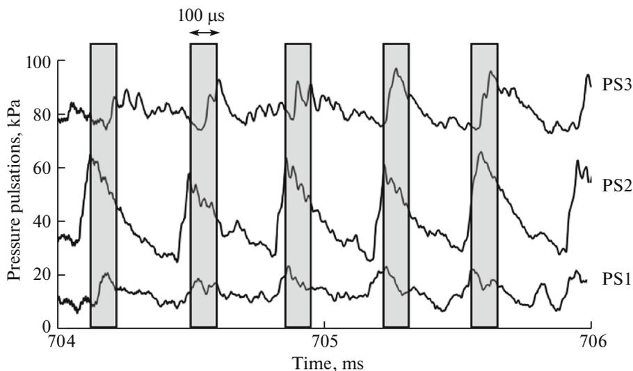
Fig. 4. Readings of the pressure pulsation sensors.
