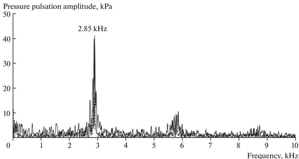
Fig. 3. Fourier analysis of a fragment of the readings of the pressure pulsation sensors.
