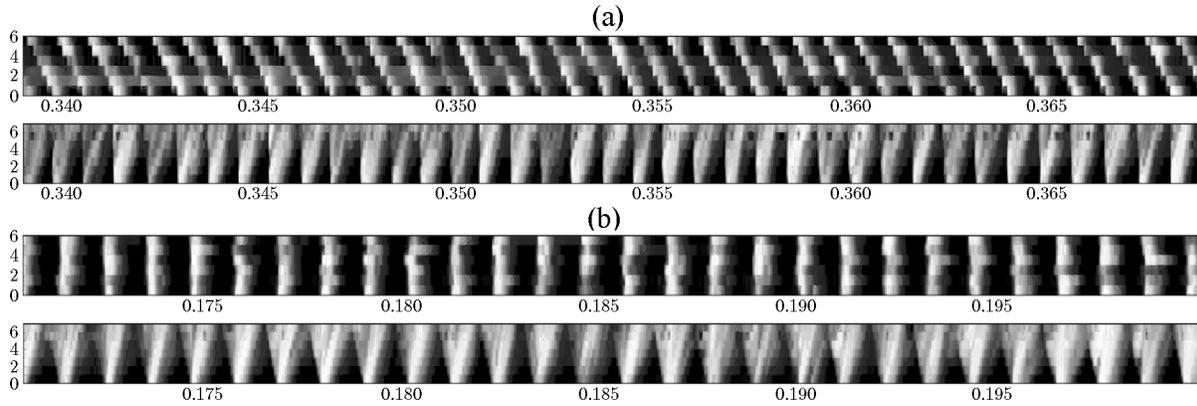
**Fig. 3.** Examples of “visualization” of signals recorded by the ionization probes in experiments with continuous spin detonation (a) and longitudinally pulsating detonation (b) regimes.
