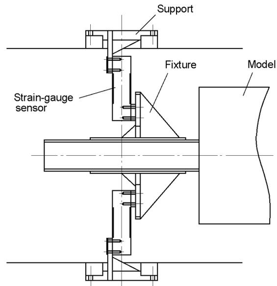
**Fig. 2.** System for measuring the thrust force generated by the detonation ramjet model.
