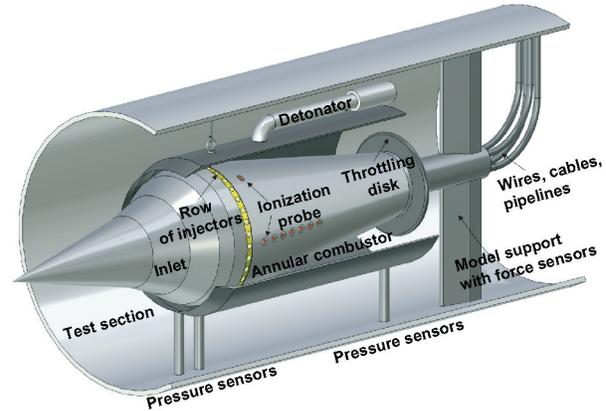
**Fig. 1.** Detonation ramjet model mounted in the wind tunnel.
