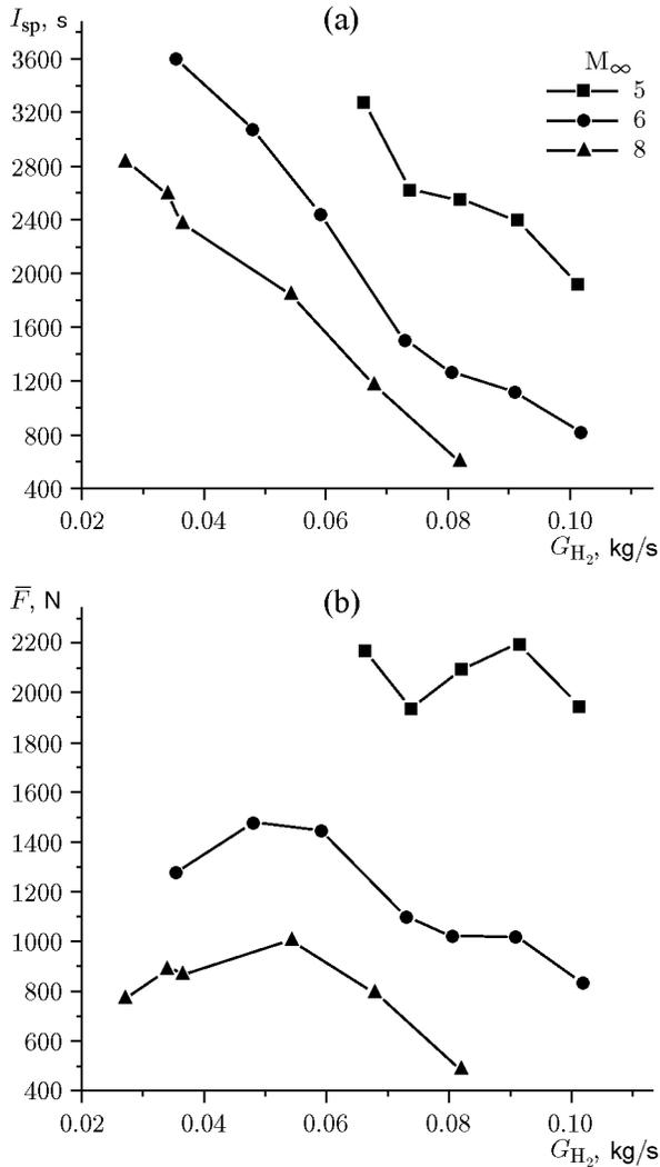
**Fig. 5.** Measured fuel-based specific impulse (a) and mean thrust (b) generated by the detonation ramjet model versus the mass flow rate of hydrogen for  $M_\infty = 5, 6,$  and  $8$ .
