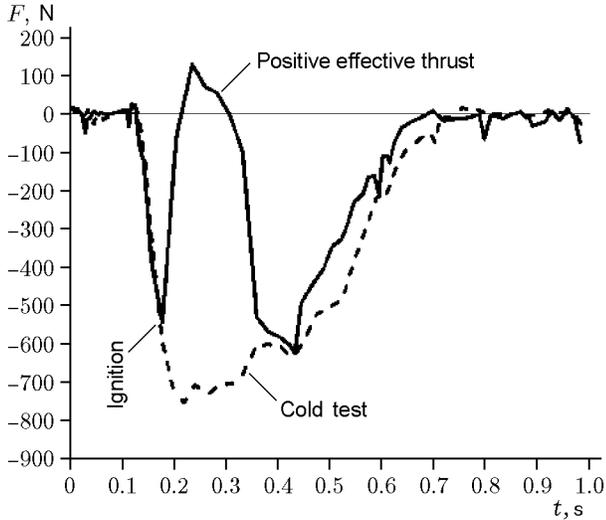
**Fig. 4.** Measured instantaneous force acting on the model versus time in the “hot” test ( $G_{\text{H}_2} = 0.034$  kg/s; solid curve) and “cold” test ( $G_{\text{H}_2} = 0.023$  kg/s; dashed curve) at  $M = 8$  with the D220 throttling disk.
